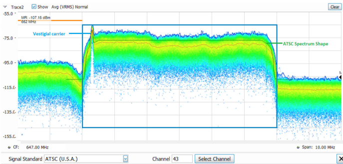
In this illustration, a single region has been selected. Since we have declared this to be an ATSC video signal, the spectrum mask for the ATSC signal is shown overlaid in the region. The signal is a close match to the spectrum mask, including the vestigial carrier at the lower side of the signal, characteristic of ATSC broadcasts.
